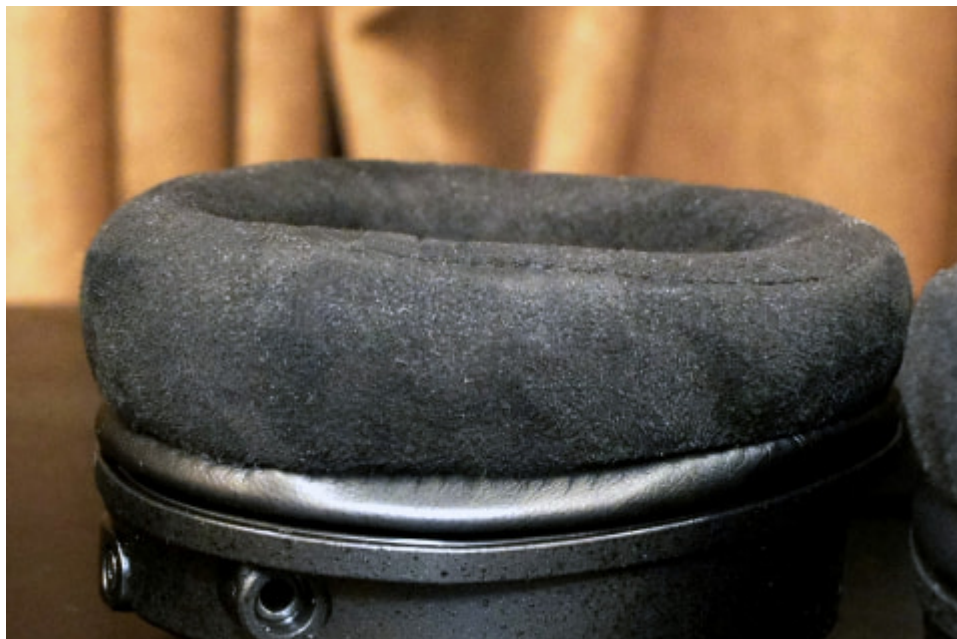
CZ-8A housing (side-view). The picture shows that the thickness on the left side is increased.
